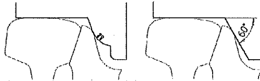
Fig. 66-Template "1W" and grinding template
