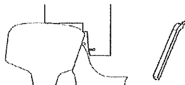
Fig. 64-Template "1H" and feeler gauge
